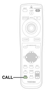
Information on the input signal source, etc., can be displayed.
